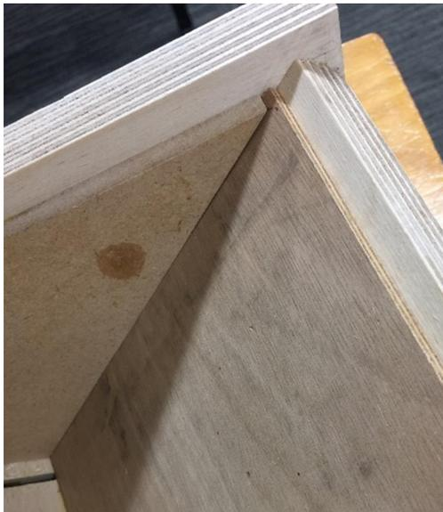
Finally, **Tony Clark** showed us his improved mitre-key cutting jig with a sacrificial insert; a standard ninety-degree V-shape with a 3mm plywood false side creating a slot to lock a replaceable piece of plywood inside the end of the jig.
